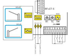
[Example 2]. Control N.C. 1-6 (safety stop) can be changed into control N.O. 1-4 (closing) setting  $6\rightarrow 4=0$  FF.
