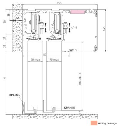
The VALOR T automation wall fixing measurements are illustrated in the diagram, considering that the door wing profiles are not of our production.
