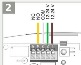
Connect the wires accordingly:
