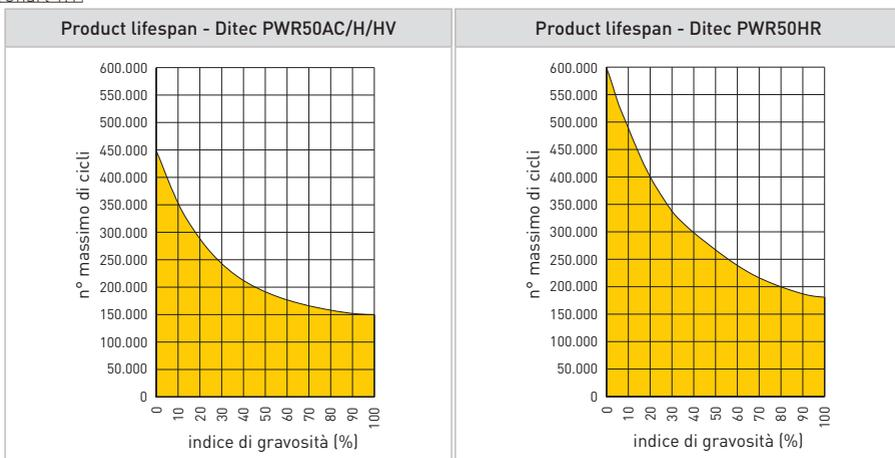
The chart below shows an example of an operating unit lifespan calculation:
