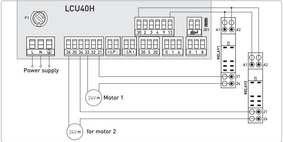
**i** **NOTE:** the relays are supplied with PWR50HR motors.
