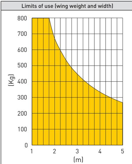
The product lifespan is conditioned by the extent of other onerous conditions: with reference to Tab. 1.1, various corrective factors have been assessed in relation to the weight and width of the wing and the usage conditions; when taken as a whole, they affect the lifespan of the operating unit (see Chart 1.1).
