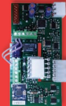
plug-in electronic card compatible with all Entrematic control panels
