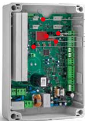
**2 plug-in slots for control** and radio safety cards
